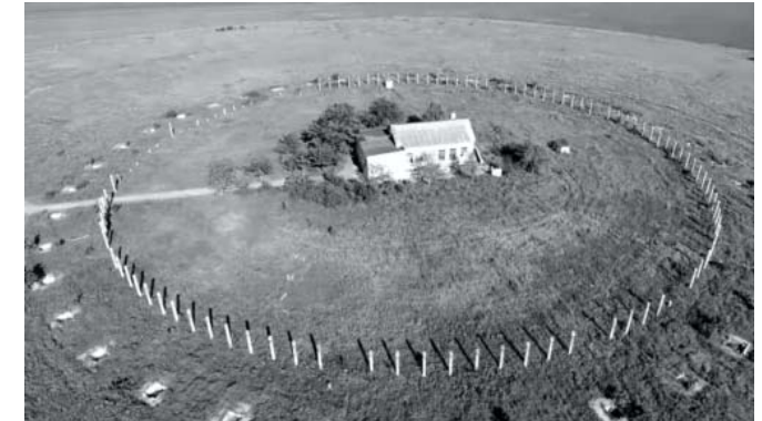
High frequency direction finding (via Google) – or circularly disposed aerial array (CDAA)
