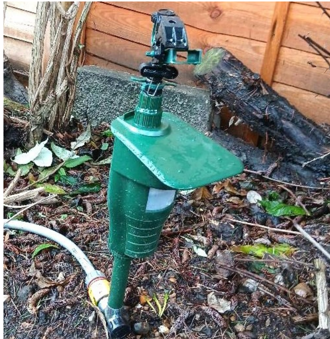
Finally the solution arrived in the form of the German-made 'Wasser-Tierabwehr'. This gizmo senses the fox and spurts a harmless arc of water in their direction whilst at the same time making a mechanical noise that acts as a secondary deterrent - pic by author.
